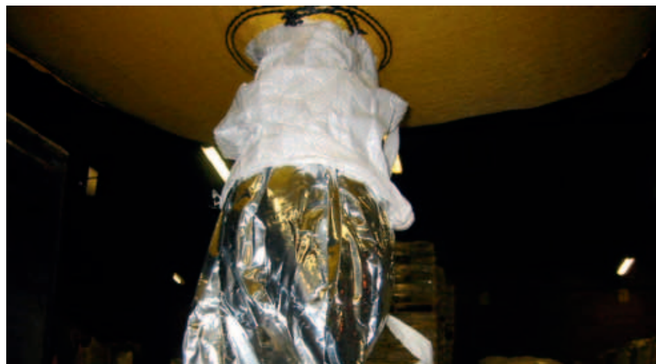
BigBag discharge spout showing aluminium lining.
